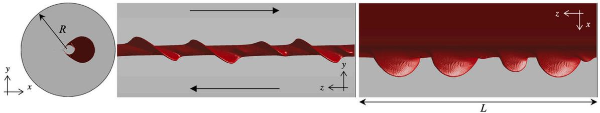
Fig. 10. Crack pattern for  $\nu = 0.45$  and  $K_{III}/k_{IIIc} = 3.92$  in the large model with  $R = 40l_c$  and  $L = 200l_c$  (with  $g_c/(El_c) = 1$ ).
