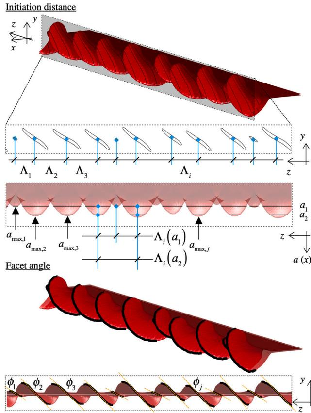
Fig. 5. Schematic illustration of the method used to measure the initiation distance between neighboring facets and the facet angle (with a model size of  $R = 20l_c$  and  $L = 200l_c$  and material parameters  $g_c/(El_c) = 1$  and  $\nu = 0.37$ ).
