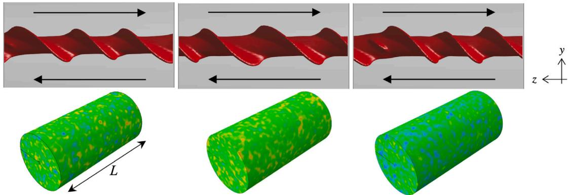
Fig. A.22. Effect of different random  $g_c$  distributions on the crack pattern.
