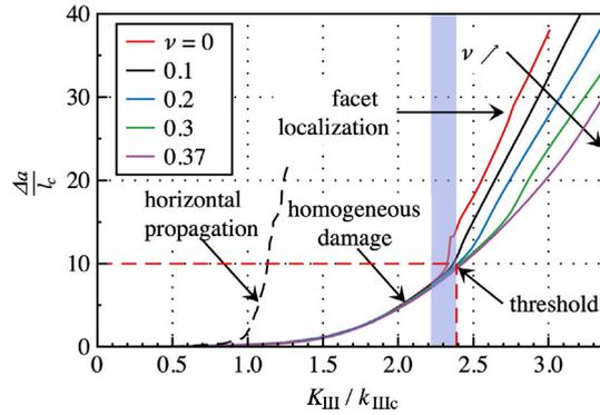
Fig. 15. Normalized relative crack advancement as a function of the normalized loading. The period, where facets start to localize is highlighted in blue. The results for the case with no energy decomposition is displayed with the black dashed curve.
