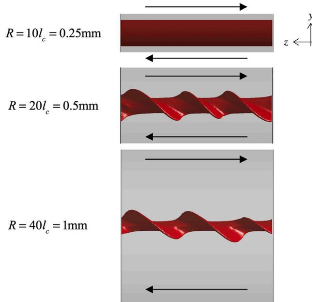
Fig. A.23. Effect of model size  $R$  on the crack pattern.
