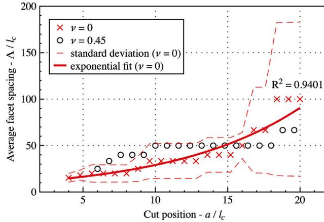
Fig. 13. Evolution of normalized facet distance as a function of the position of the cutting plane for a fixed loading. The dashed lines represent the standard deviation. The measured values are fitted with the exponential function:  $\Lambda/l_c = ae^{\beta \frac{a}{l_c}}$ . The model dimensions were  $R = 40l_c$  and  $L = 200l_c$ .
