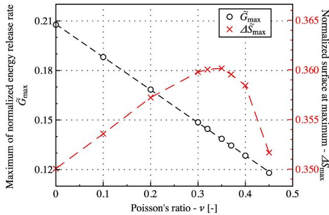
Fig. 18. Maximum of the normalized energy release rate and the related normalized surface opening as a function of Poisson's ratio for  $\phi = 45^\circ$ . The curves are guide to the eye.
