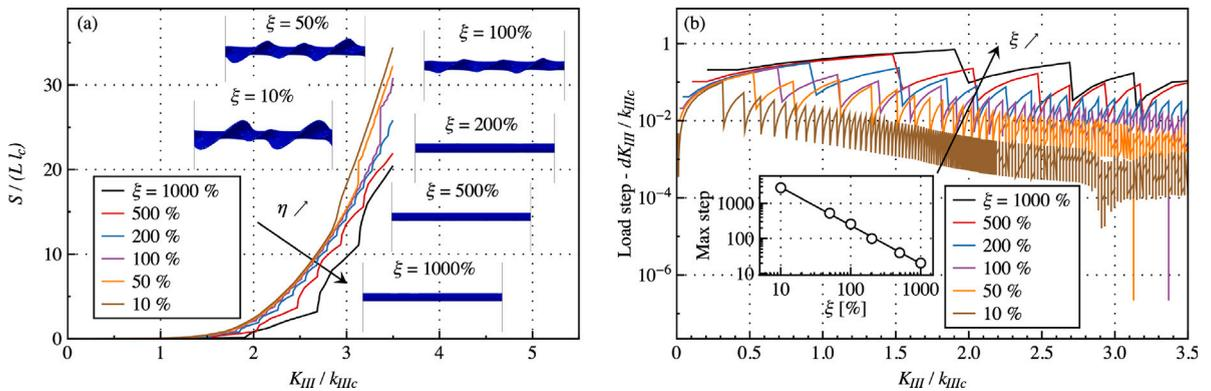
Fig. A.25. Impact of load step control on (a) crack pattern and (b) load step. The inset displays the iterations required to achieve  $K_{III}/k_{IIIc} = 2.54$ .
