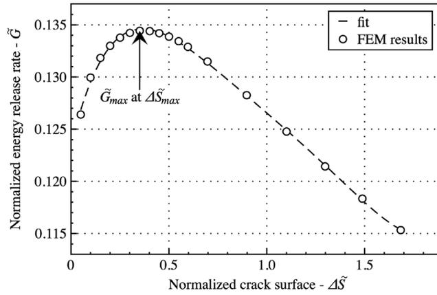
Fig. 17. Normalized incremental energy release rate as a function of normalized crack opening for  $\nu = 0.37$ . The arrow points to the maximum value  $\tilde{G}_{max}$  at the normalized surface opening  $\Delta\tilde{S}_{max}$ .
