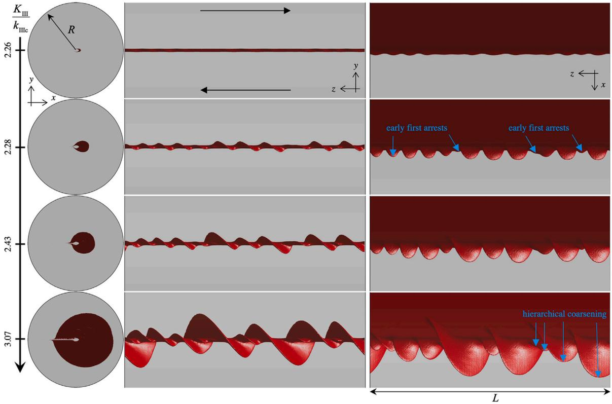
Fig. 9. Crack evolution for increasing  $K_{III}/k_{IIIc}$  in the large model with  $\nu = 0$ ,  $R = 40l_c$  and  $L = 200l_c$  (with  $g_c/(El_c) = 1$ ).
