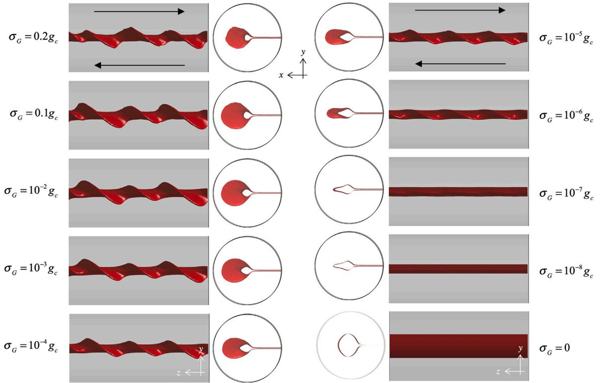
Fig. A.21. Effect of variation in fracture toughness ( $\sigma_G$ ) on the crack pattern for the same loading.
