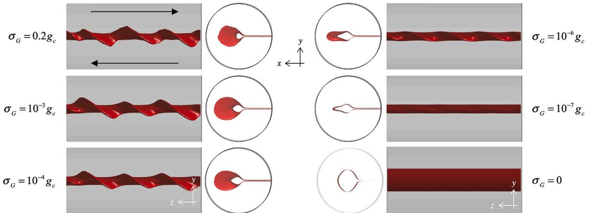
Fig. 6. Effect of GRF variation ( $\sigma_G$ ) on the crack pattern for the same loading with  $l_G = l_c$ . The simulation domain dimensions were  $L = 80l_c$  and  $R = 20l_c$  with material parameters  $g_c/(El_c) = 1$  and  $\nu = 0.37$ .
