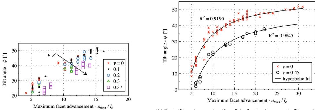
(a) Facet tilt angle as a function of crack advancement and Poisson's ratio in fitted with the hyperbolic function:  $\phi(a_{max}) = \frac{\phi_{max}}{a_{max}/l_c} + \phi_{max}$ , where  $\phi_{max}$  denotes the facet angle on the plateau. Results are plotted from various loading stages in the model with  $R = 40l_c$  and  $L = 200l_c$ .
