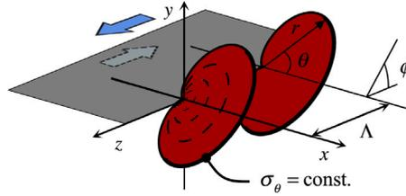
Fig. 16. Idealized crack shape illustrating the coupled criterion, with the applied coordinate system.
