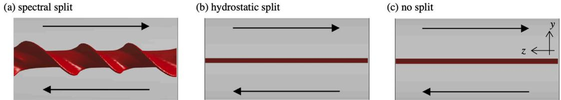
Fig. 8. Effect of different energy decomposition schemes on the crack pattern (with a model size of  $R = 20l_c$  and  $L = 80l_c$  and material parameters  $g_c/(El_c) = 1$  and  $\nu = 0.37$ ).
