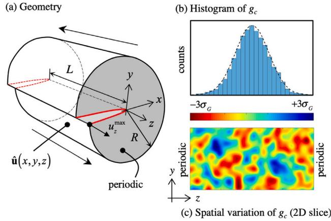
**Fig. 3.** (a) The geometry and boundary conditions of the phase-field model are depicted. (b) The histogram shows the variation applied by the Gaussian random field (GRF) used to induce facets in the model. (c) A 2D example of the GRF is also shown. Both the abscissa of the histogram and the color bar are scaled between  $-3\sigma_G$  and  $+3\sigma_G$ .
