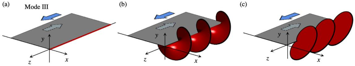
Fig. 2. Mode III crack front segmentation: (a) Problem definition; (b) continuous formation; (c) abrupt facet emergence. The mother crack is displayed in gray, while the facets are shown in red. The blue arrows show the direction of the macroscopic shear applied in the  $yz$  plane.
