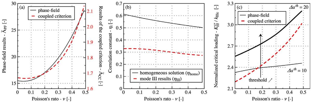
Fig. 20. (a) Normalized initiation distance; (b) correlation constant  $\eta_i$ ; and (c) critical loading as a function of Poisson's ratio.
