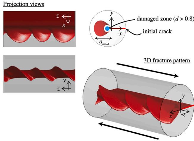
Fig. 4. Typical crack pattern obtained from the phase-field model under antiplane shear. The red surface in the figure corresponds to the isosurface<sup>3</sup> of the damage variable at  $d = 0.8$ , with a model size of  $R = 20l_c$  and  $L = 80l_c$  and material parameters  $g_c/(El_c) = 1$  and  $\nu = 0.37$ .
