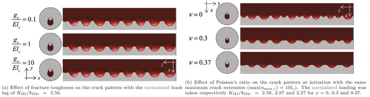
Fig. 11. Effect of material properties on the crack pattern at initiation with  $R = 20l_c$  and  $L = 200l_c$ .
