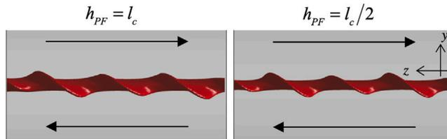
Fig. A.24. Effect of finite element mesh size on the crack pattern.
