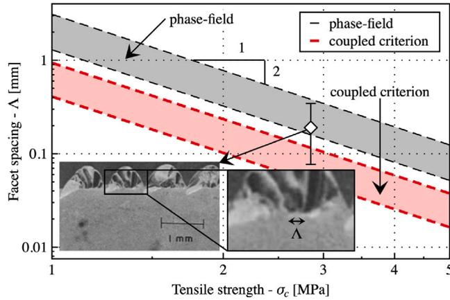
Fig. 19. Characteristic initiation distance between neighboring facets as a function of tensile strength in double logarithmic scale. The numerical results are shown for a range of material properties ( $E = 3.00\text{--}4.14$  MPa,  $\nu = 0.45$ ,  $g_{\text{mat}} = 67.8\text{--}113.0$  J/m<sup>2</sup>). Experimental results shown in the inset are taken from Knauss (1970). The error bars represent 95% percentiles.
