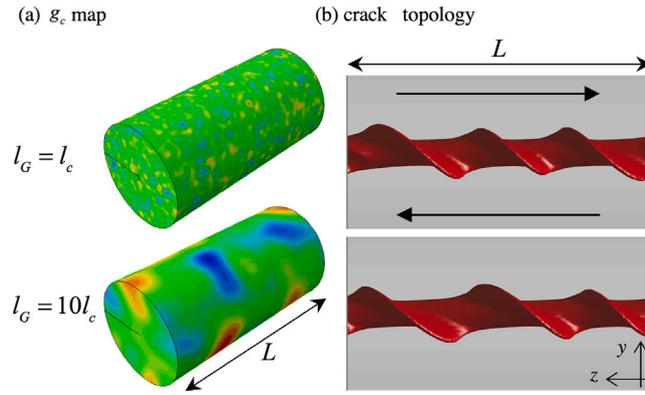
Fig. 7. Effect of GRF length scale on the crack pattern with the same random seed. (a)  $g_c$  map corresponding to  $\sigma_G = 10^{-3}g_c$ . The colors in the figure represent a variation of approximately  $-3\sigma_G$  to  $+3\sigma_G$ . The GRF is displayed with  $l_G = l_c$  on the top and  $l_G = 10l_c$  on the bottom. (b) Corresponding phase-field crack patterns with  $g_c/(El_c) = 1$  and  $\nu = 0.37$ . The simulation domain dimensions were  $L = 80l_c$  and  $R = 20l_c$ .
